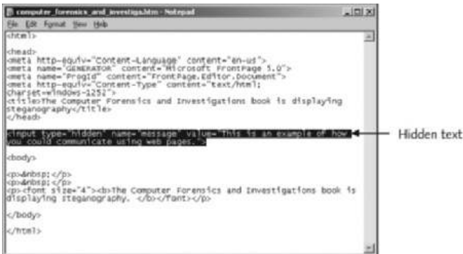
Figure 8-24 The HTML code reveals hidden text Courtesy of Microsoft Corporation
