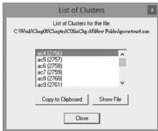
Figure 8-10 Viewing all clusters used by the gametour4.exe file
